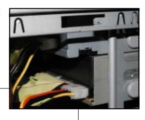
7. Make sure that the drive and bay holes align as shown. When in place, the drive protrudes about an inch from the front panel.
